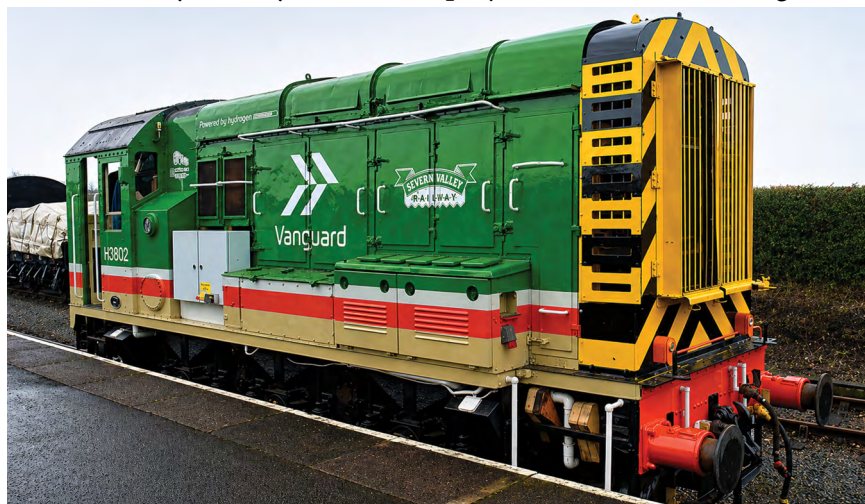
Figure 1. HydroShunter hydrogen-battery hybrid locomotive developed by Vanguard, demonstrating high-efficiency operation for shunting duties through integration of fuel cell technology and onboard energy storage, enabling significant reductions in emissions, noise, and fuel consumption.
